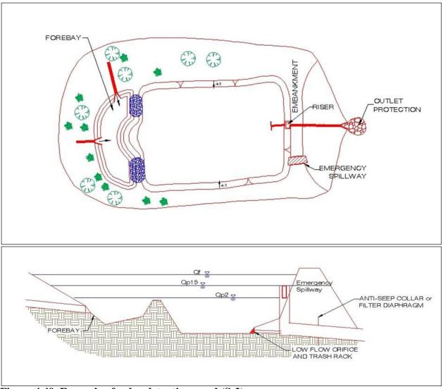
Figure 4.49 Example of a dry detention pond (S-2).
