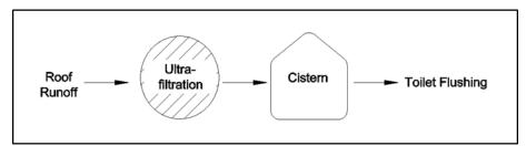
Figure 2. Example 2 treatment schematic.
