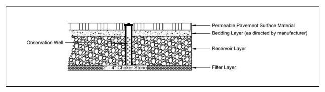
Figure 4.14. Cross-section of an enhanced permeable pavement design without an underdrain.
