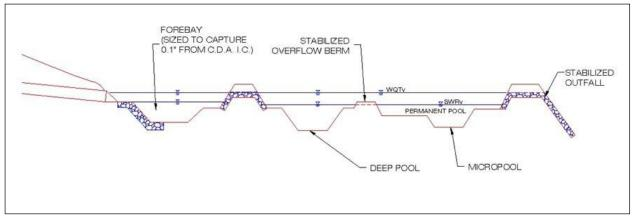
Figure 4. 54 Cross section of a typical stormwater wetland.
