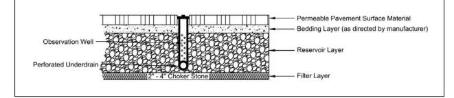
Figure 4.12. Cross-section of a standard permeable pavement design.
