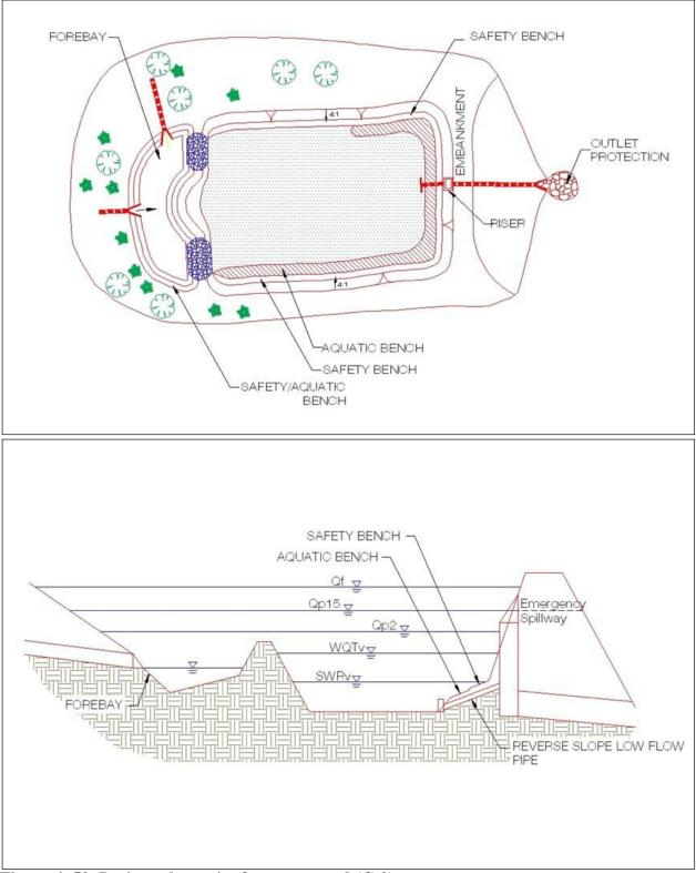
Figure 4. 50 Design schematics for a wet pond (C-2).
