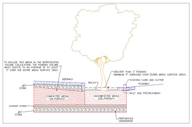
Figure 4.9. Example design of a tree box with compacted media extending below sidewalk.
