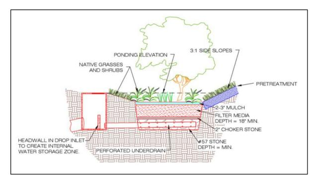
Figure 4.3. Example bioretention design with internal water storage (IWS).
