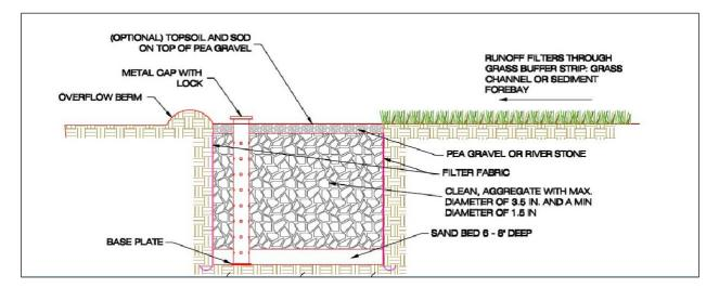
Figure 4.17. Example design of an infiltration trench.
