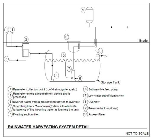
Figure 4.24. Example of a rainwater harvesting system detail.
