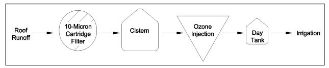
Figure 1. Example 1 treatment schematic.
