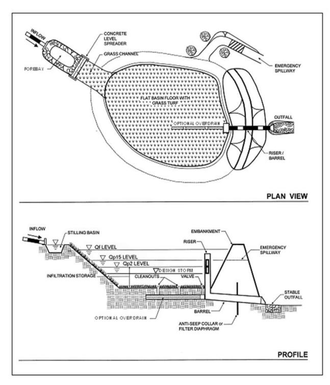
Figure 4.19. Example design of an infiltration basin.
