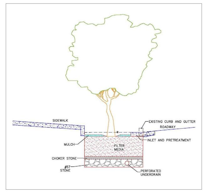
Figure 4.8. Example design of a tree box.
