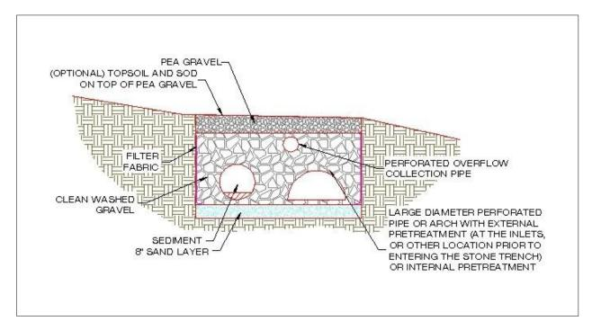
Figure 4.18. Example design of an infiltration practice with supplemental pipe storage.
