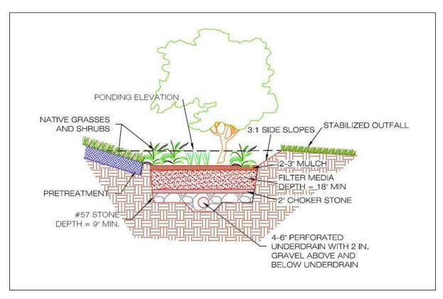
Figure 4.4. Example standard bioretention design.
