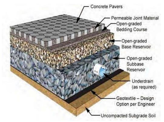
Figure 4.11. Cross-section of permeable pavement (source: ICPI).
