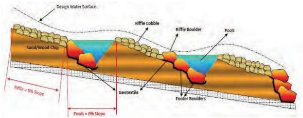
Figure 4.37. Example of Regenerative Stormwater Conveyance (O-4).
