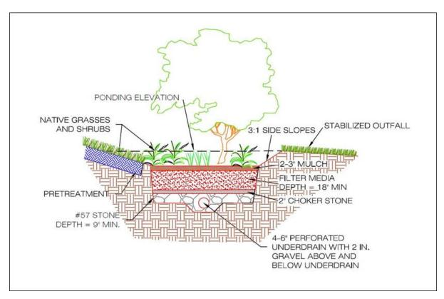
Figure 4.4. Example standard bioretention design.
