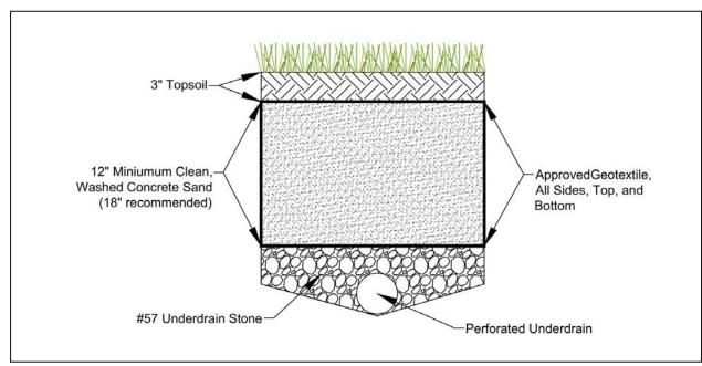
Figure 4.39. Typical schematic for a nonstructural or surface sand filter (note: material specifications are found in Table 4.44).
