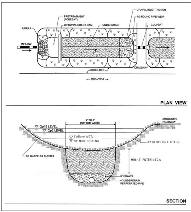
Figure 4.35. Example of a dry swale/bioswale (O-2).
